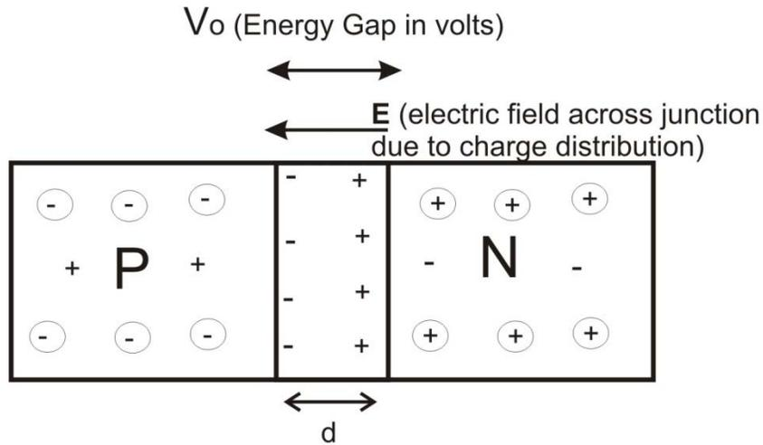
In p type materials, negative acceptor ions are fixed and holes are mobile.
