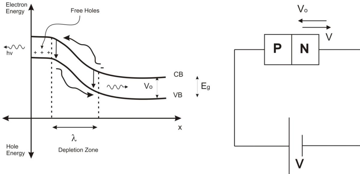
Gap  $V_0$  is reduced to  $V_0 - V$  since applied voltage from battery lowers barrier
